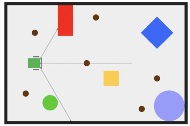
For this task you should use sensors with which the robot should navigate through the room. Your robot has 3 infrared sensors with which it can measure the distance from itself to walls or other obstacles. You can see the sensors drawn in the simulation environment by the three lines that lead away from the robot. The infrared sensors have the following numbers: sensor left 4, sensor middle 5, sensor right 6.
